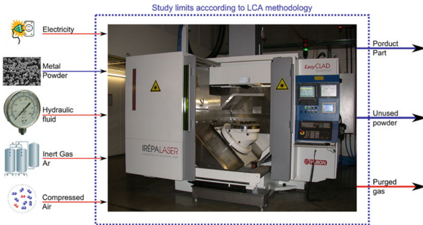
Fig. 17 Directed energy deposition (CLAD) process
